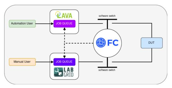
As mentioned in above diagram, FC will use different frameworks' interface to disconnect all frameworks' access to DUT by default. Then, FC will monitor the job queue of different frameworks, if find some framework's job pending on any resource, FC will connect the resource again to that framework. With that way, no conflict will be occured.
