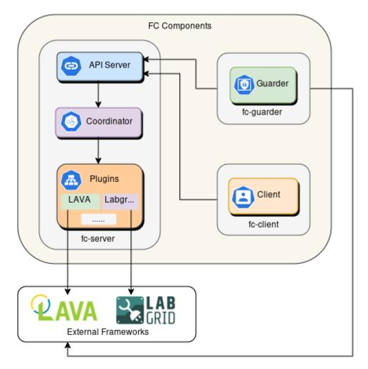
See above diagram, FC has three main components inside, fc-server, fc-client and fc-guarder:
